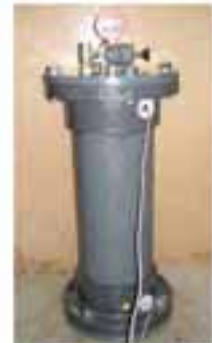
Fig. 2 - Photo of UofS2 portable pressure column to evaluate formwork pressure
