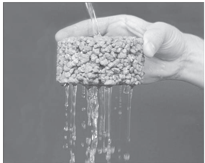
Figure 1. Pervious concrete cylinder showing water passing through
