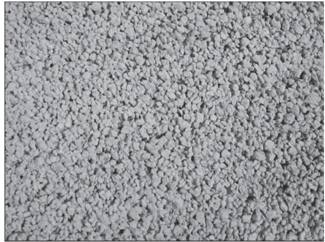
Figure 4. Typical top surface of hardened pervious concrete
