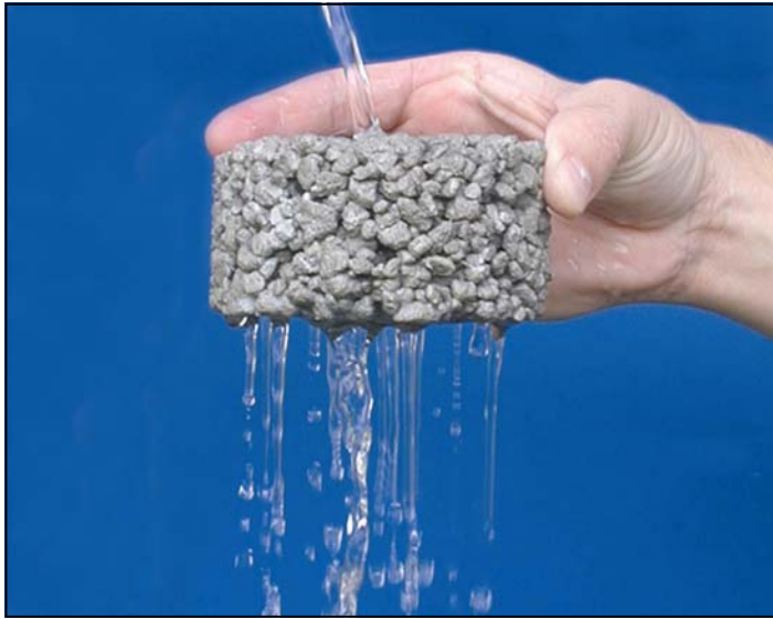
Figure 3. Pervious concrete has between 15 and 25% voids that allow stormwater to percolate through it.
