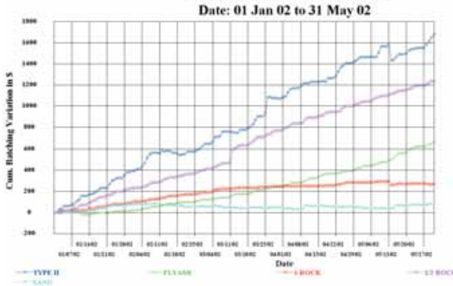
Figure 2. Significant Reduction in Material Over-Batching After Installation of Improved QC System (five plants producing a total of 300,000 yd 3 for that period)
