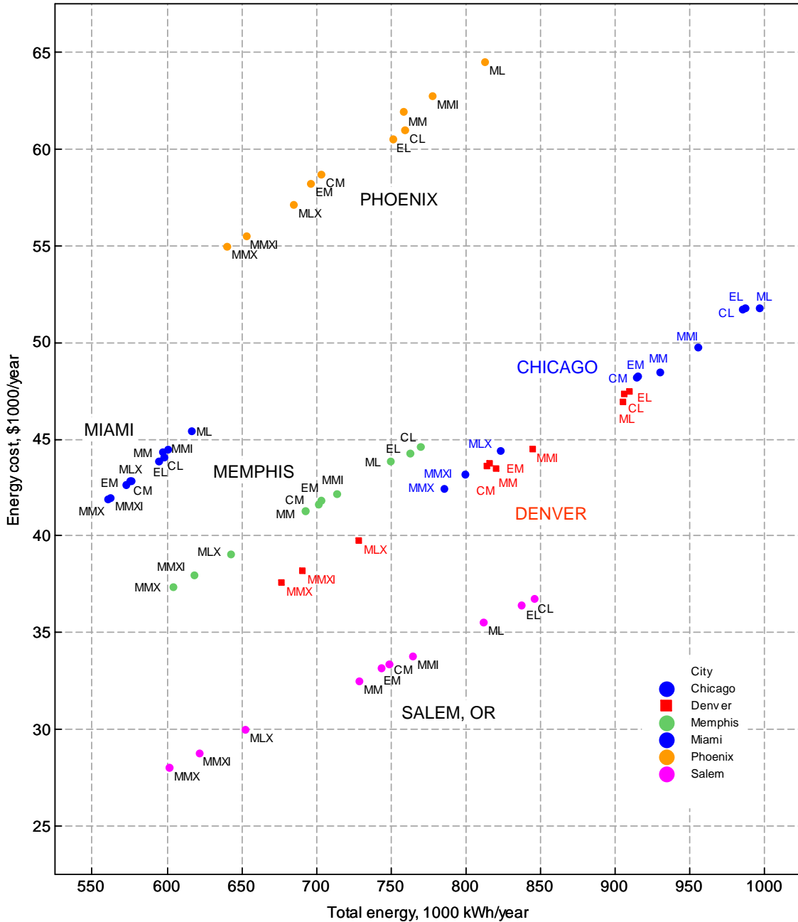
FIGURE 1 - THE RELATIONSHIP BETWEEN ANNUAL ENERGY USE AND COST VARIES BY CITY. SEE TABLE 1 FOR AN EXPLANATION OF THE BUILDING DESIGNATION ABBREVIATION
