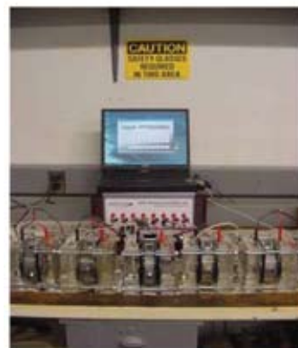
Fig. 1: ASTM C 1202 (RCP) test setup and suggested qualitative indicators in the test method
