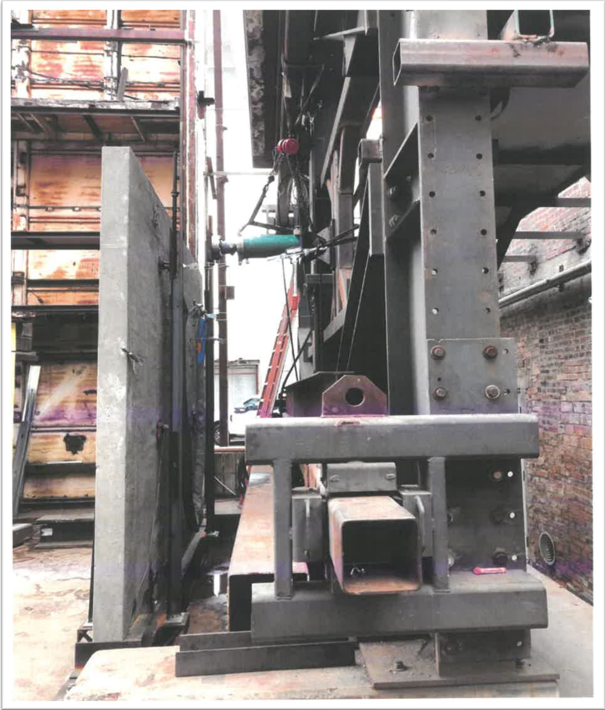
Figure 7. One of the compressive specimens tilted for testing
